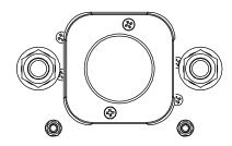
2-M10 Load Wiring 2-M10 10-12N.m Torque 10-12N.m
